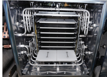
Hot-zone and retort. Use to shelves to support the parts produced by metal injection moulding (MIM)
